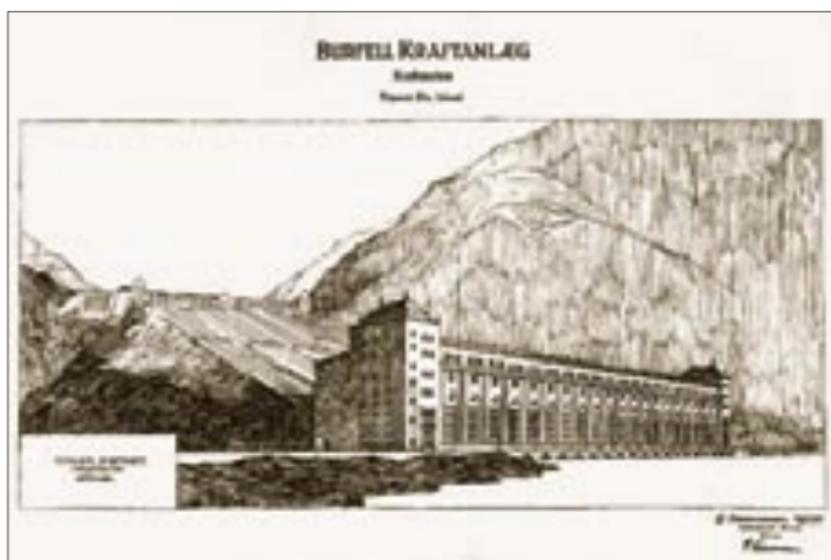
to produce electricity which would mainly be utilized for fertilizer production. He envisaged five stations on Thjórsá from the Urridafoss falls and upriver beyond Búrfell, as well as a station at Hrauneyjafoss on the River Tungnaá. Búrfell would have been by far the largest station. The plan was to dam Thjórsá at Klofaey and divert the water through an open channel into Bjarnarlón and to an intake dam at Sámstadaklif.
