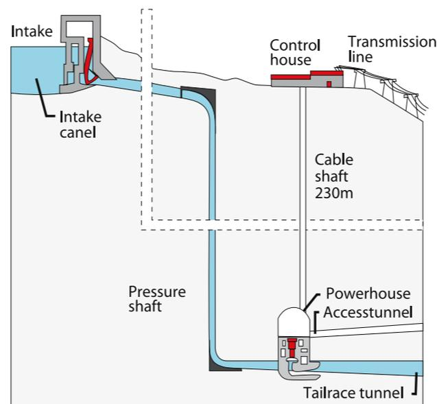
A 132 kV double circuit transmission line links the Blanda power station to the national grid 12 km to the north. Electricity production by the Blanda station is remote-controlled via optical cable and microwave link from a dispatch centre in Reykjavík. Station personnel, engineers and electricians, are primarily responsible for maintenance and supervision.
